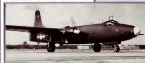
▲ Second XP4M-1 Aircraft 02790 was the second Mercator prototype. The J33 jet engine air intake is below the propeller, in the open position.
